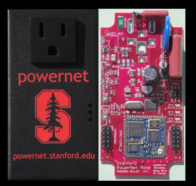
Custom-built meters Sample once per second Wireless collection of data Ease of deployment
