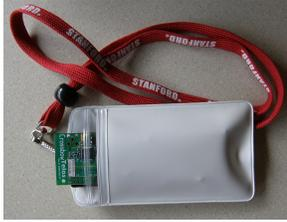
Figure 1: Each participant in the deployment received a TelosB mote inside a white pouch. Subjects wore the motes around their necks using a lanyard.
