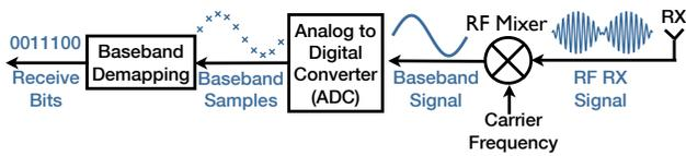
Figure 1: Simplified block diagram of an RF Receiver
