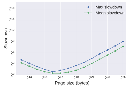
Figure 5: Mean and maximum slowdown relative to optimal page size for a range of transfer sizes between 4 KB and 32 MB.
