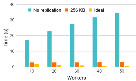
Figure 3: Performance of the dynamic replication mechanism, which improves performance by over 11× on a network-intensive sparse lookup workload.
