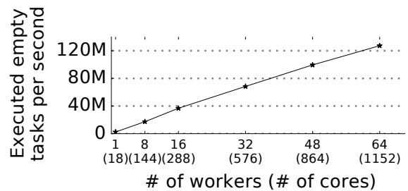
Figure 11: The task rate of Canary grows linearly with the number of cores, reaching more than 120 million tasks per second on 1,152 cores, because every core spawns and executes tasks in parallel.
