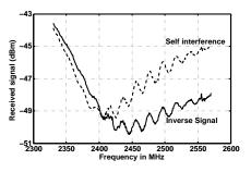
Figure 17: Frequency response of a previous version of our balun circuit. The frequency selective mismatch, caused by poor layout, prevented balun cancellation beyond 25 dB.
