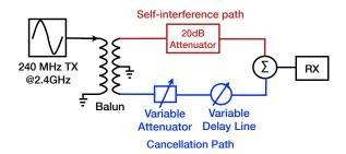
Figure 4: Wired setup to measure the cancellation performance of signal inversion vs phase offset. The phase offset experiment uses an RF splitter instead of a balun to split the signal.
