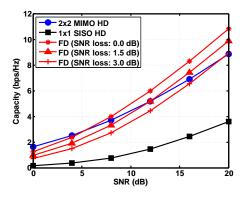
Figure 16: Capacity comparison of the proposed full duplex system and the  $2 \times 2$  MIMO half duplex system
