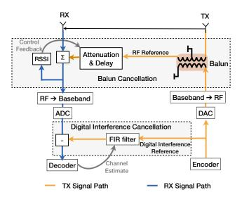
Figure 3: Block diagram of full duplex system. The ideal cancellation setup uses passive, high precision components for attenuation and delay adjustment.
