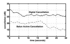
Figure 14: Performance of balun active cancellation and of digital cancellation over time. Before cancellation, the received power is -45dBm for the balun active cancellation experiment, and -58dBm for digital cancellation. Once tuned, the QHx220 settings are stable for over 10 seconds. The 20 dB maximum is caused by the nonlinearities of the QHx220. Digital cancellation performance, on the other hand deteriorates within a span of 3-4 seconds and needs more frequent tuning.
