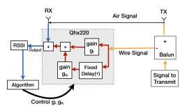
Figure 7: Block diagram of full duplex system with Balun Active Cancellation. The RSSI values represent the energy remaining after cancellation. Our algorithm adapts attenuation parameters ( $g_i$  and  $g_q$ ) to minimize this energy.
