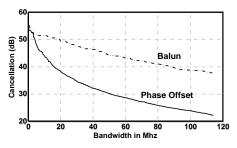
Figure 6: Cancellation performance with increasing signal bandwidth when using the balun method vs using phase offset cancellation.
