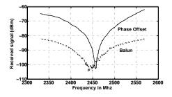
Figure 5: Cancellation of the self-interference signal with the balun vs with phase offset. The received signal is -49dBm without any cancellation. Using a balun gives a flatter cancellation response.
