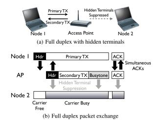
Figure 9: The full duplex MAC protects primary and secondary transmissions from losses due to hidden terminals. A busytone is used to protect periods of single-ended data transfer.
